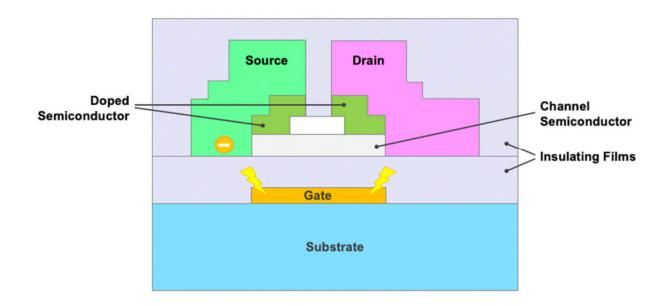
is a depiction of a typical TFT, which includes a source, drain, and a gate:
