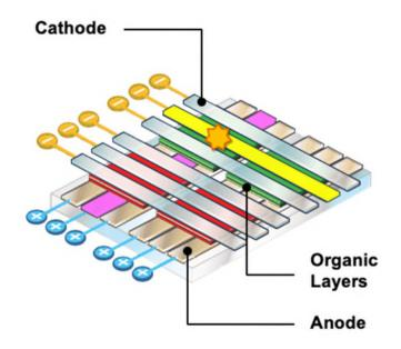
42. In active matrix OLEDs, the anode layer is instead divided up into individual pixels and overlaps a thin film transistor ("TFT") matrix. The TFT matrix itself is circuitry that determines which pixels are turned on, resulting in faster refresh rates and the consumption of less power, which is ideal for high-resolution displays like TVs and smartphones. The following is an illustration of an active matrix OLED:
