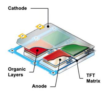
43. An active matrix OLED panel has a matrix of pixel circuits, with one circuit driving each of the OLED pixels. Each pixel circuit in the matrix contains multiple TFTs. The following
