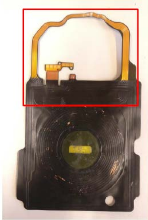
Flex Printed Circuit Extracted from Samsung Galaxy S8 (Magnetic Secure Transmission ("MST") coil identified)
