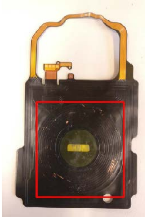
Flex Printed Circuit Extracted from Samsung Galaxy S8 (wireless power coil identified)
