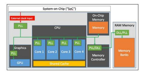
44. Modern SoC processors often also use additional system memory, which is provided as an external memory chip or module and interfaces with the processor through the processor's on-chip memory controller. The stylized figure above also shows an exemplary external memory module. Although there are many kinds of external memory that may be used,
