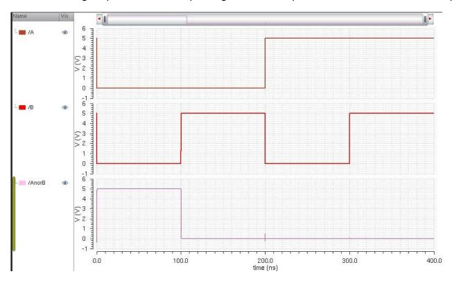
For the NOR gate pin 25 is +5V and pin 20 ground. The inputs are 26 and 27 (A and B), output pin is 28
