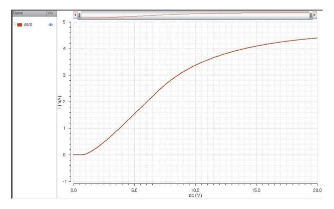
The pins for the NMOS are as follow; pin 33 source, pin 34 gate, pin 35 drain and the body is grounded that's why there is no pin. This the IV curve Id vs VGS
