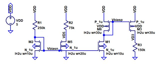
2. To model a mismatch in a threshold voltage between M1 and M2 a small-valued voltage source may be put at the gate of M2 as seen below. Using LTspice simulations show, and discuss in your own words, how threshold voltage influences the currents in the basic current mirror. (2 points)
