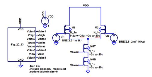
2. What is the input CMR for the following diff-amp? What is the allowable (so that all transistors stay in the saturation region) range of the output voltage? Finally, what is the output voltage (DC + AC). Verify your hand calculations using LTspice. (4 points)
