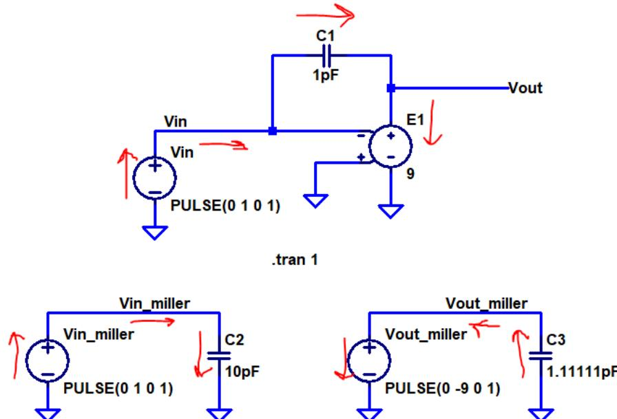
2. Estimate the frequency response of the following amplifier. Verify your hand calculations using LTspice (4 points)
