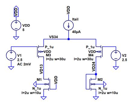
2. Determine the AC and DC currents and voltages in the following circuit. Use LTspice to verify your hand calculations. (3 points)
