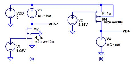
3. Repeat problems 1 and 2 but replace the 1mV AC source with a 1mV peak sinusoid at 1 kHz (no new hand calculations). Re-simulate to verify your answers using an LTspice transient simulation. (2 points, 0.5 points for each simulation)
