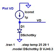
2. Estimate, using hand calculations, the reference voltage and reference voltage's temperature coefficient in the following circuit. Compare your answer to an LTspice simulation. (4 points)
