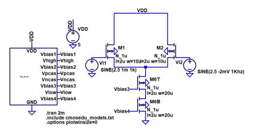
2. What is the input CMR for the following diff-amp? What is the allowable (so that all transistors stay in the saturation region) range of the output voltage? Finally, what is the output voltage (DC + AC). Verify your hand calculations using LTspice. (4 points)
