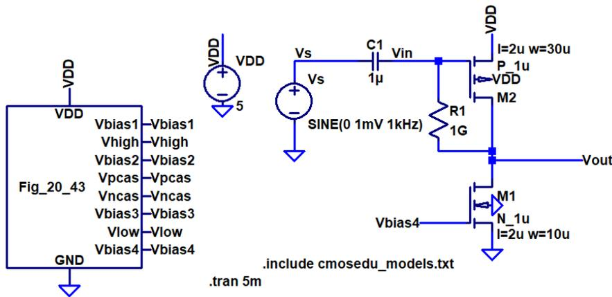
3. Replace the current-source load transistors in the above schematics with a 100k resistor and determine the output voltage, both DC and AC. Verify your answers with LTspice. (4 points)
