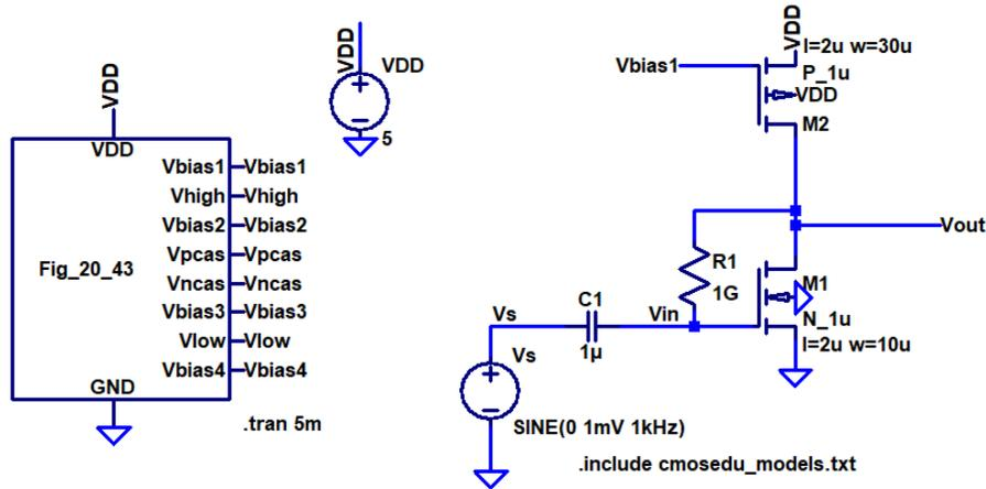
2. Determine the AC and DC currents and voltages in the following CS amplifier. Verify your hand calculations using LTspice (3 points)
