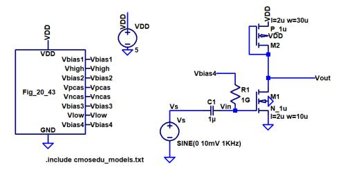
2. Determine the AC current and voltages in the following circuit. Verify your hand calculations using LTspice (3 points)
