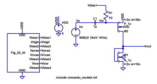
3. Replace the gate-drain connected transistors in the above schematics with a 100k resistor and determine the output voltage, both DC and AC. Verify your answers with LTspice. (4 points)
