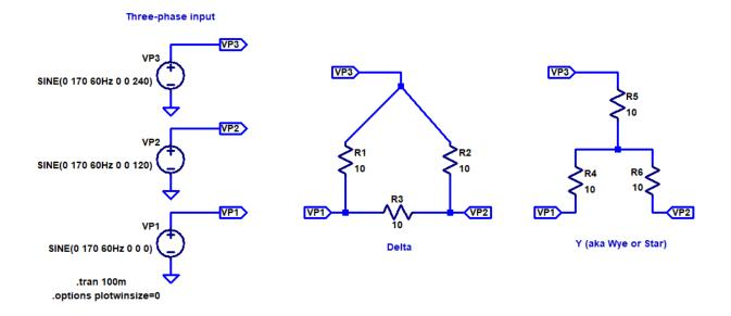
2. For each of the circuits seen below determine the apparent power ( $I_{RMS}V_{RMS}$ ) dissipated by the resistor. Verify yours answer using LTspice. (8 points)
