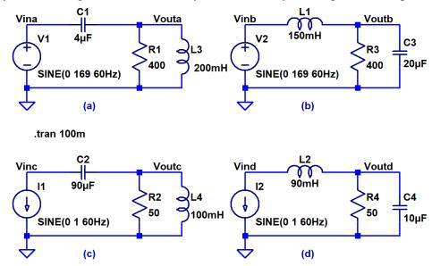
2. Re-draw the schematics in problem 1 with the input sources labeled as phasors and representing the capacitors and inductors using complex numbers (see Fig. P7.62 on page 452 of the book for example). (2 points)
