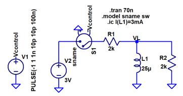
Note that the initial current through the inductor is NOT zero.
