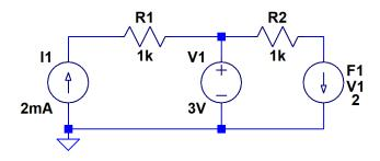
4. Find the Thevenin equivalent of the following circuit at the port indicated by the red dots. (10 points)
