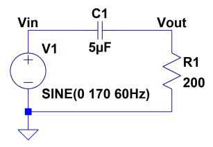
6. Find Vout in the following circuit and sketch on the same plot with Vin, showing the phase shift and magnitude. (15 points)
