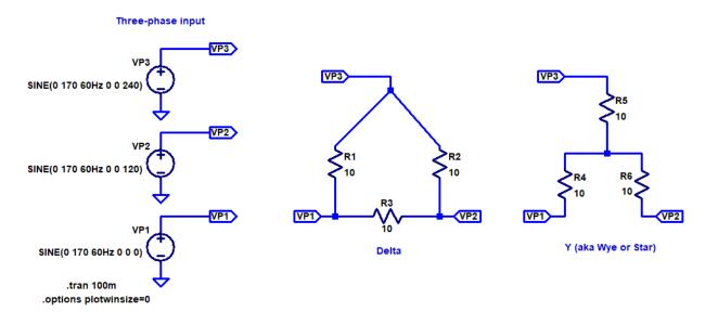
2. For each of the circuits seen below determine the apparent power ( $I_{RMS}V_{RMS}$ ) dissipated by the resistor. Verify yours answer using LTspice. (8 points)
