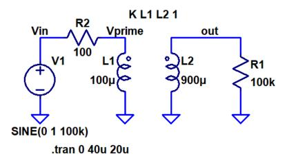
2. What is the average power delivered to R1 in the above circuit? Verify your answer using LTspice. Compare to the power supplied by Vin. Where does the difference go in the circuit (what else heats up?). (3 points)
