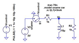
Note that the initial current through the inductor is NOT zero.
