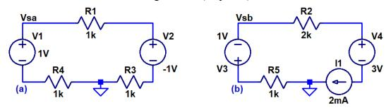
2. Find V1 and V2 in the following circuit using mesh analysis. (10 points)
