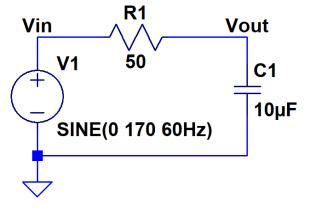
6. Find Vout in the following circuit and sketch on the same plot with Vin, showing the phase shift and magnitude. (15 points)
