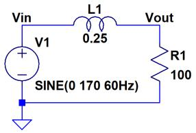
7. Find Vout in the following circuit and sketch in the time-domain, along with Vin, showing the phase shift and magnitude. (20 points)
