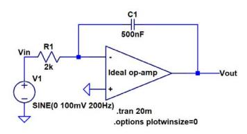
2. Find the output voltage for each of the following circuits using AC analysis (as always make sure your hand calculations are concise and clear). Sketch the output voltage and input voltage on the same plot in the time domain and compare to LTspice. Again, as in question 1, you may have to remove the DC signal in the output to properly compare your AC hand calculations to simulation results. (8 points)
