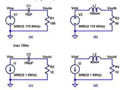
3. Re-draw the schematics in problem 2 with the input sources labeled as phasors and representing the capacitors and inductors using complex numbers (see Fig. P7.62 on page 452 of the book for example). (2 points)
