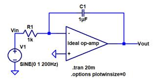
2. Find the output voltage for each of the following circuits using AC analysis (as always make sure your hand calculations are concise and clear). Sketch the output voltage and input voltage on the same plot in the time domain and compare to LTspice. Again, as in question 1, you may have to remove the DC signal in the output to properly compare your AC hand calculations to simulation results. (8 points)
