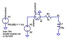
Note that the initial current through the inductor is zero.
