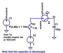
3. Write the equations describing the voltage across the capacitor, Vc, in the following circuits for both the rising and falling edges of the input pulse. Again, use LTspice to verify your answer. (4 points)
