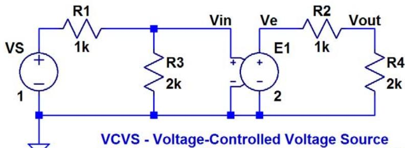
**VCVS - Voltage-Controlled Voltage Source**
