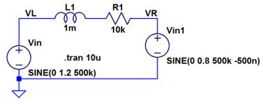
4. Write equations for Vout in each of the following circuits and then sketch the output voltage and current in each circuit against time. Verify with LTspice.
