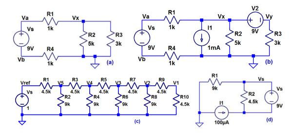
2. Determine the currents and voltages in the following circuits using both superposition and mesh analysis. Verify your hand calculations using LTspice. (6 points)
