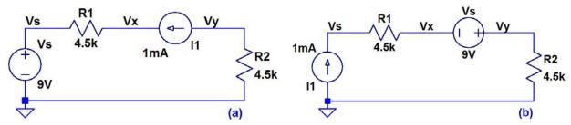
2. Find the voltages Vs and Vx and the current through R2 in each of the following circuits. Verify your hand calculations using LTspice. (6 points)
