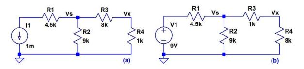
3. **Using superposition** show how to find Vx in the following circuits. Verify your hand calculations using LTspice. (6 points)
