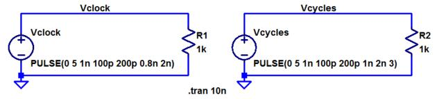
6. Suppose you are doing a sim where you need a clock signal operating at 1 MHz that oscillates between 0 V and 5 V. Assume the duty cycle of the clock is 50% (the clock signal is high [= 5 V] the same amount of time that the clock is low [= 0V]). Assume the rising and falling edges are 10 ns. Show how to implement this clock signal in LTspice. (2 points)
