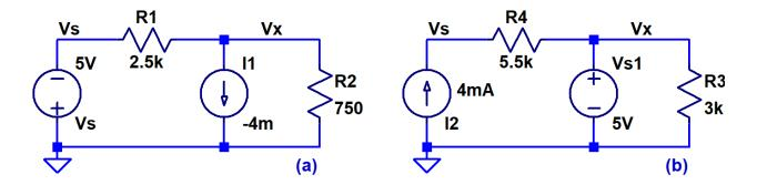
2. Find the voltages Vx and Vs and the current through Vs in each of the following circuits. Verify your hand calculations using LTspice. (6 points)
