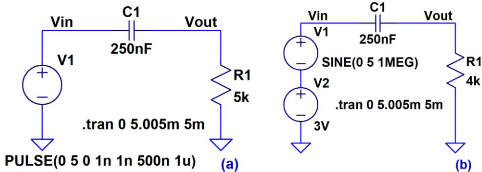
2. Determine  $V_{out}$  for each of the following circuits. Sketch  $V_{out}$  and  $V_{in}$  on the same plot. Show your hand calculations for credit. Verify your answers using LTspice. (8 points)
