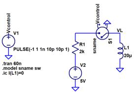
Note that the initial current through the inductor is zero.
