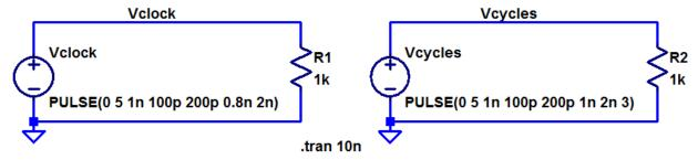
6. Suppose you are doing a sim where you need a clock signal operating at 10 MHz that oscillates between 0 V and 5 V. Assume the duty cycle of the clock is 50% (the clock signal is high [= 5 V] the same amount of time that the clock is low [= 0V]). Assume the rising and falling edges are 10 ns. Show how to implement this clock signal in LTspice. (2 points)
