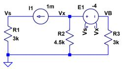
3. Find Vout in the following circuit. For all intents and purposes you can assume the gain of the VCVS is infinite. (3 points)
