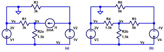
3. For the circuits in problem 2 find the Thevenin and Norton equivalent circuits from Vx to ground (with R2 in the circuit). Show that you get the same value for Vx that you calculated in problem 2 with your equivalent circuits for both Thevenin and Norton equivalent circuits. Verify your Thevenin and Norton circuits are correct using LTspice. (4 points)
