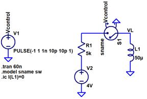
Note that the initial current through the inductor is zero.
