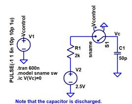
3. Write the (2) equations describing the voltage across the capacitor, Vc, in the following circuit for both the rising and falling edges of the input pulse. Again, use LTspice to verify your answer. (3 points)
