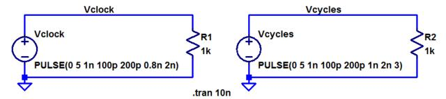
6. Suppose you are doing a sim where you need a clock signal operating at 25 MHz that oscillates between 0 V and 2 V. Assume the duty cycle of the clock is 50% (the clock signal is high [= 2 V] the same amount of time that the clock is low [= 0V]). Assume the rising and falling edges are 10 ns. Show how to implement this clock signal in LTspice. (2 points)
