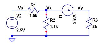
4. Using mesh analysis find the voltage Vx in the following circuit. (20 points)
