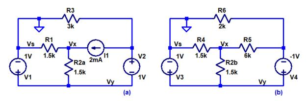
3. For the circuits in problem 2 find the Thevenin and Norton equivalent circuits from Vx to ground (with R2 in the circuit). Show that you get the same value for Vx that you calculated in problem 2 with your equivalent circuits for both Thevenin and Norton equivalent circuits. Verify your Thevenin and Norton circuits are correct using LTspice. (4 points)
