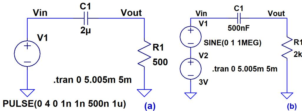
2. Determine  $V_{out}$  for each of the following circuits. Sketch  $V_{out}$  and  $V_{in}$  on the same plot. Show your hand calculations for credit. Verify your answers using LTspice. (8 points)
