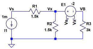
3. Find Vout in the following circuit. For all intents and purposes you can assume the gain of the VCVS is infinite. (3 points)
