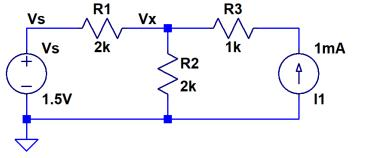
3. Find the voltage Vx in the circuit seen below. Then find the Thevenin equivalent circuit, with R2 removed, at the terminals marked by dots. Show that your Thevenin circuit is correct by comparing the value you calculated for Vx to the one you get when you put R2 across the terminals of your Thevenin equivalent. (20 points)
