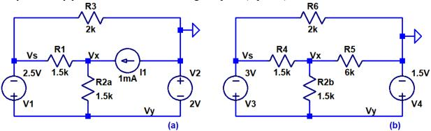
3. For the circuits in problem 2 find the Thevenin and Norton equivalent circuits from Vx to ground (with R2 in the circuit). Show that you get the same value for Vx that you calculated in problem 2 with your equivalent circuits for both Thevenin and Norton equivalent circuits. Verify your Thevenin and Norton circuits are correct using LTspice. (4 points)
