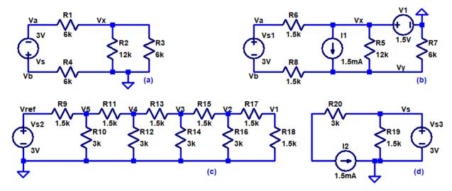
2. Determine the currents and voltages in the following circuits using both superposition and mesh analysis. Verify your hand calculations using LTspice. (6 points)
