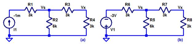
3. **Using superposition** show how to find Vx in the following circuits. Verify your hand calculations using LTspice. (8 points)
