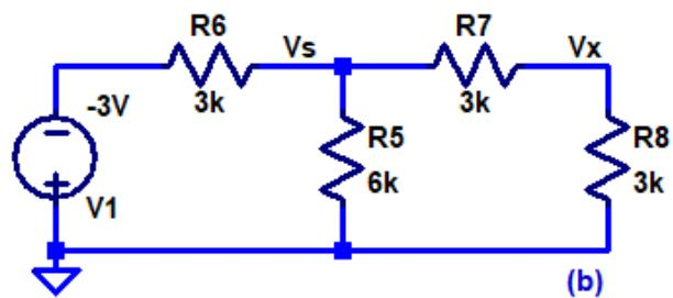
3. Using superposition show how to find  $V_x$  in the following circuits. Verify your hand calculations using LTspice. (8 points)
