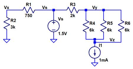
4. Write, using a text editor, the spice netlist for the circuit in problem 3. Verify your netlist is correct with LTspice. (3 points)
