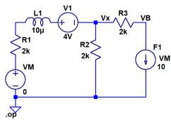
5. Calculate Vout in the following circuit. Verify your calculations using LTspice. (2 points)
