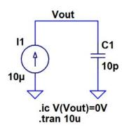
2. The following voltage, vout, is applied to a 10 pF capacitor. Plot the current through the capacitor **on this same plot** using the right side of the plot. Hint: I = C\*dvout/dt. (3 points)
