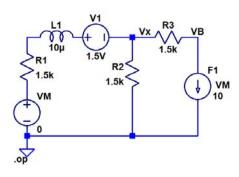
5. Calculate Vout in the following circuit. Verify your calculations using LTspice. (2 points)
