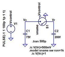
2. Plot the output of the following circuit from a time 0 to 10 ms. Assume the capacitor is initially discharged (both sides are at ground). Show your hand calculations for credit. Verify your plot with LTspice. (3 points)
